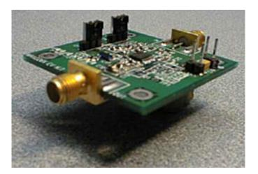
Objective: To tune and measure the cellular-band performance of this low-cost CDMA RF power amplifier.
